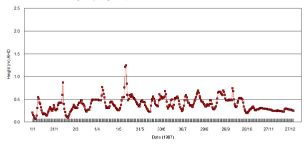
Figure 2. Water level changes in a coastal lagoon with an entrance open to coastal waters.
